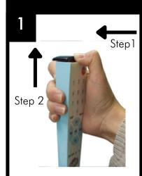
Looking at the keypad, slide the dark lens cover away from you (STEP 1) and lift the lid from the back (STEP 2).
