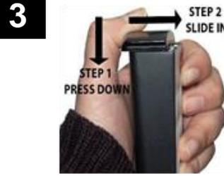
With the keypad facing away from you, close the cover by gently pressing it down (STEP 1) and sliding it until it aligns with the front (keypad) of the device (STEP 2).
