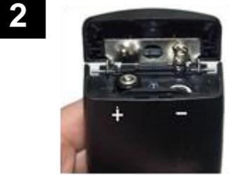
Install **2 AAA batteries**. Make sure the + and - symbols on the metal hinge of the battery compartment correspond with the + and - end of each battery.
