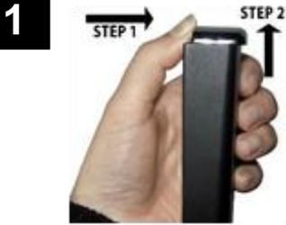
Looking at the keypad, slide the dark lens cover away from you (STEP 1) and lift the lid from the back (STEP 2).
